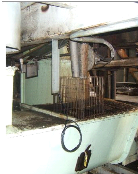
Fig. 4—The ColourQ colorimeter in situ above the wet sugar screw at Harwood Mill.
