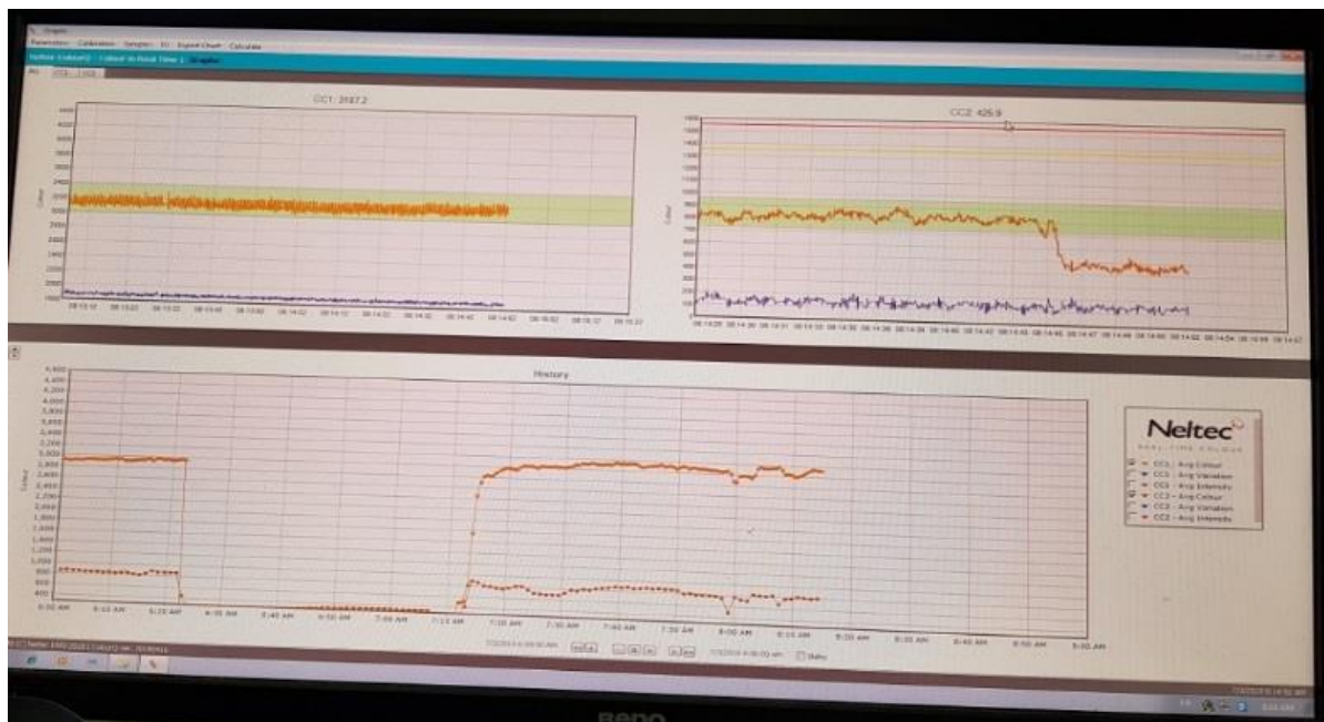
Figure 4 Graphs displaying the output signal from the Neltec transducer on the magma screw (top left), No 4 fugal (top right) as 3 minute real-time displays. The bottom display is a combined 3 hour real-time display.
