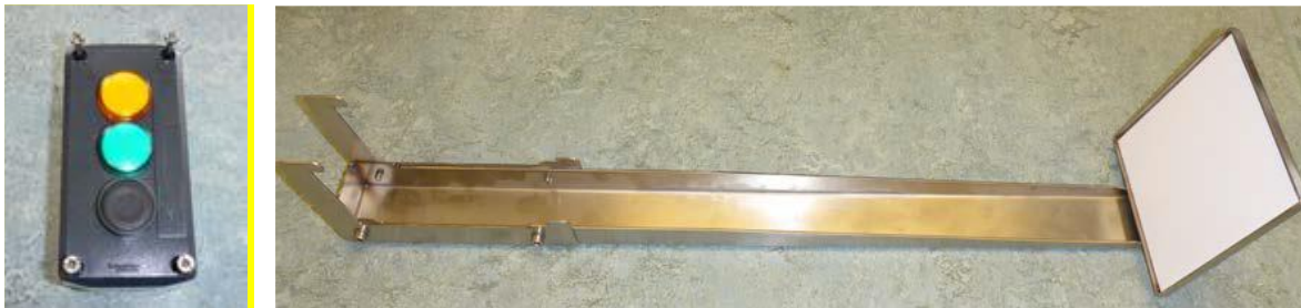
Figure 8 Button box with push button and signalling lamps, calibration arm with tile
