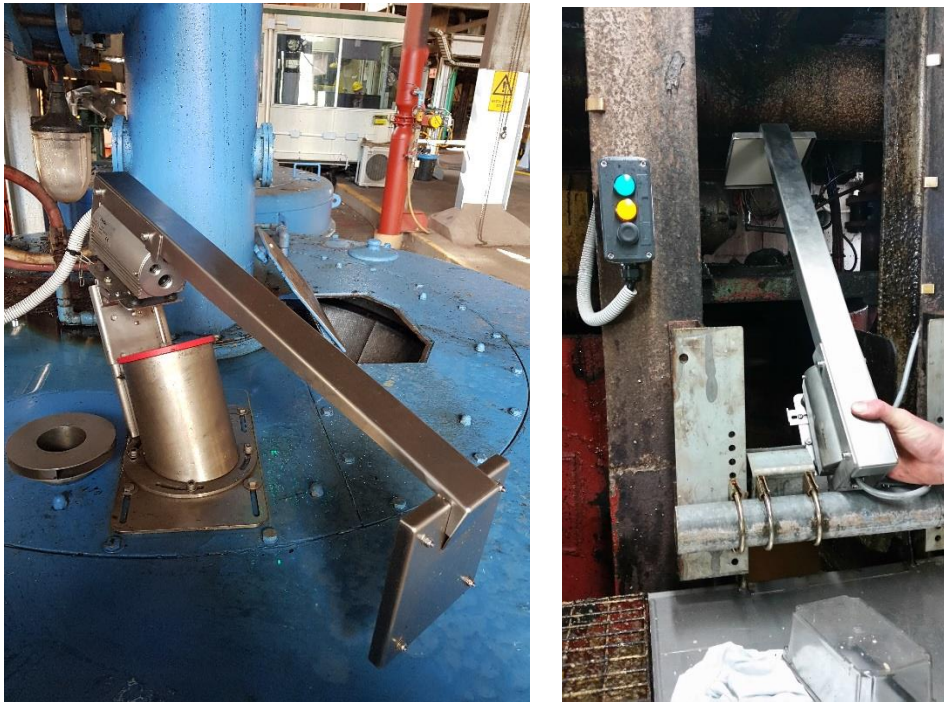
Figure 9 Positioning of the Read Head and Calibration Tile on No.4 Fugal and screw during the calibration process
