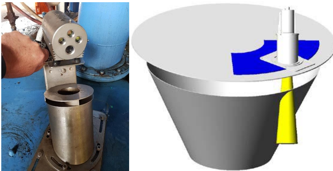
Figure 3 Layout of Neltec unit on No.4 Low Grade Fugal.
