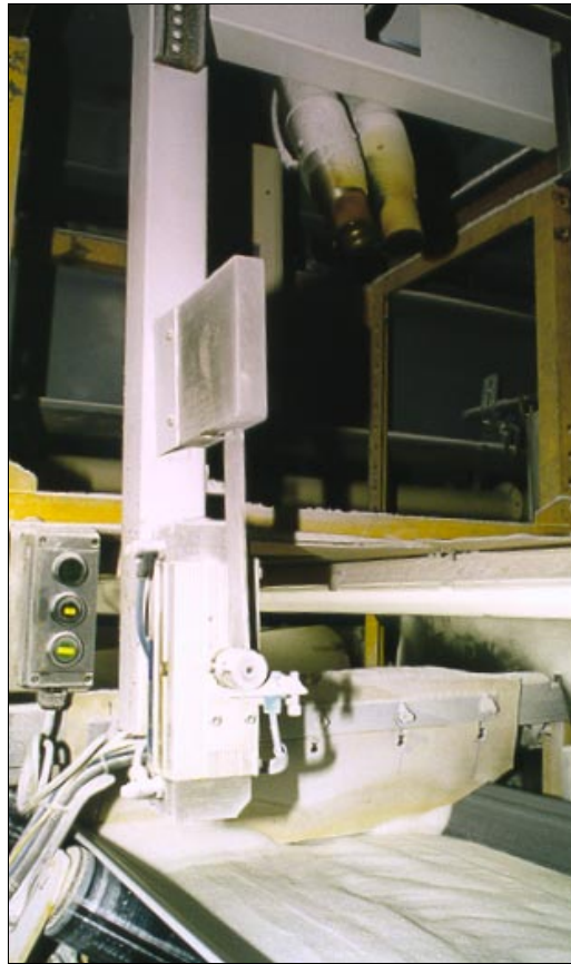
Fig. 2 Neltec ColourQ 800 installed above a conveyor belt
